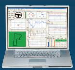
Telemetry Monitor Software enables real time viewing of data via direct serial communication, GSM modems or radio modems. Data can be viewed in various formats such as charts, bar and XY graphs, dial gauges, numerics, lights and scroll charts. All parameters are user definable.
